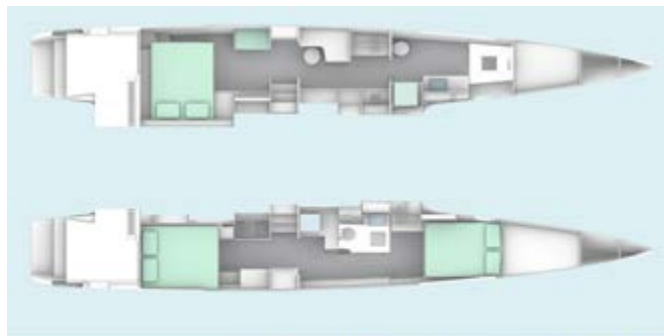
WindeLO 54 - hulls plan for nacelle with U-shaped galley 1 master cabin, 1 office and wardrobe, 1 private forward head 2 guest cabins, 1 central head, 1 central storage area
