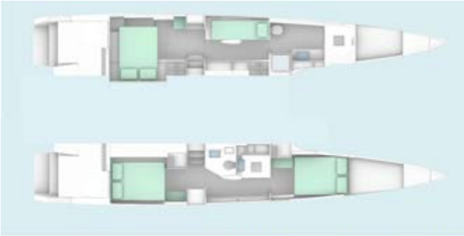
Windelo 50 - hulls plan proposition for U-shaped galley 1 master cabin, 1 retractable berth and its Saville office, 1 private forward head 2 guest cabins, 1 central head and 1 separated WC
