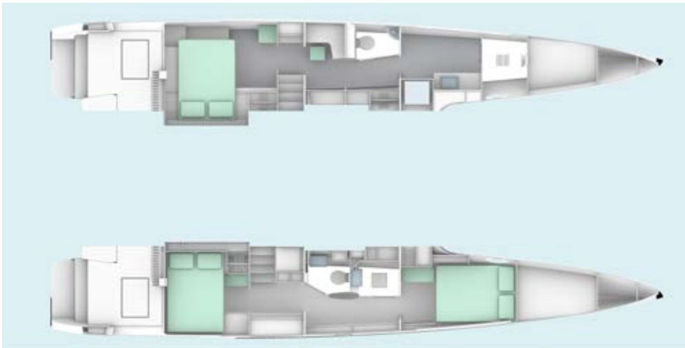
Windelo 50 - hulls plan for nacelle with L-shaped galley 1 master cabin, 1 separated WC and 1 forward head 2 guest cabins, 1 separated WC and 1 central head
