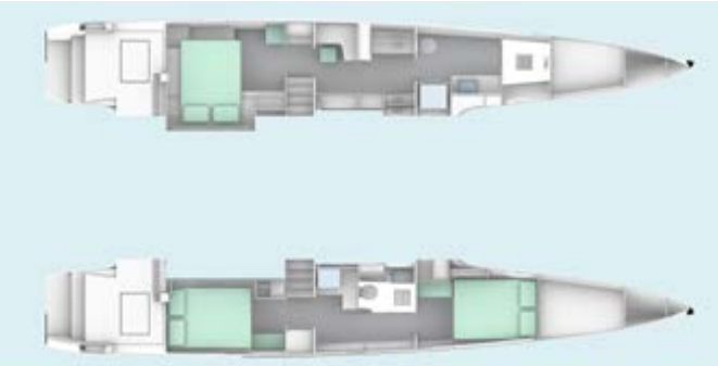
Windelo 50 - hulls plan proposition for U-shaped galley 1 master cabin, 1 office and its wardrobe, 1 private forward head 2 guest cabins, 1 central head, 1 central storage piece
