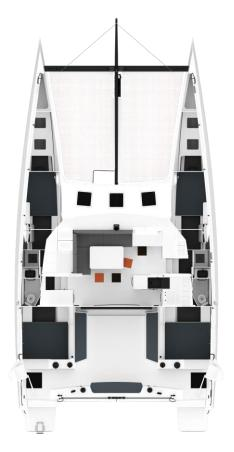
Ventilation done by two Lewmar "LP60" opening hatches (50 x 50 cm) in the roof, two Lewmar "T03" opening hatches (28 x 23 cm) in the front Plexiglas window and two flush Goïot "Luxair" opening hatches (50 x 23 cm) in the aft bulkhead windows
