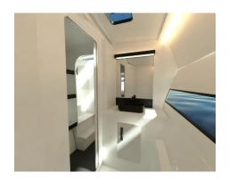
One toilet compartment with a white composite sandwich sliding and retractable door: one manual sea toilet with its black water tank, one black round sink with its black mixer faucet. One mirror with its LED lighting stripe, one cupboard under the sink with a light "Polaris" grey door. One deck opening hatch (25 x 25 cm) and one fixed hull window (120 x 18 cm). One LED lighting stripe on the ceiling
